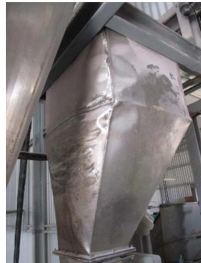
*Damage to transfer system. Left. Vacuum pump chamber and pump, PVC transfer piping and evidence of spot fires on the floor. Right. Distortion of hopper caused by explosion.*
